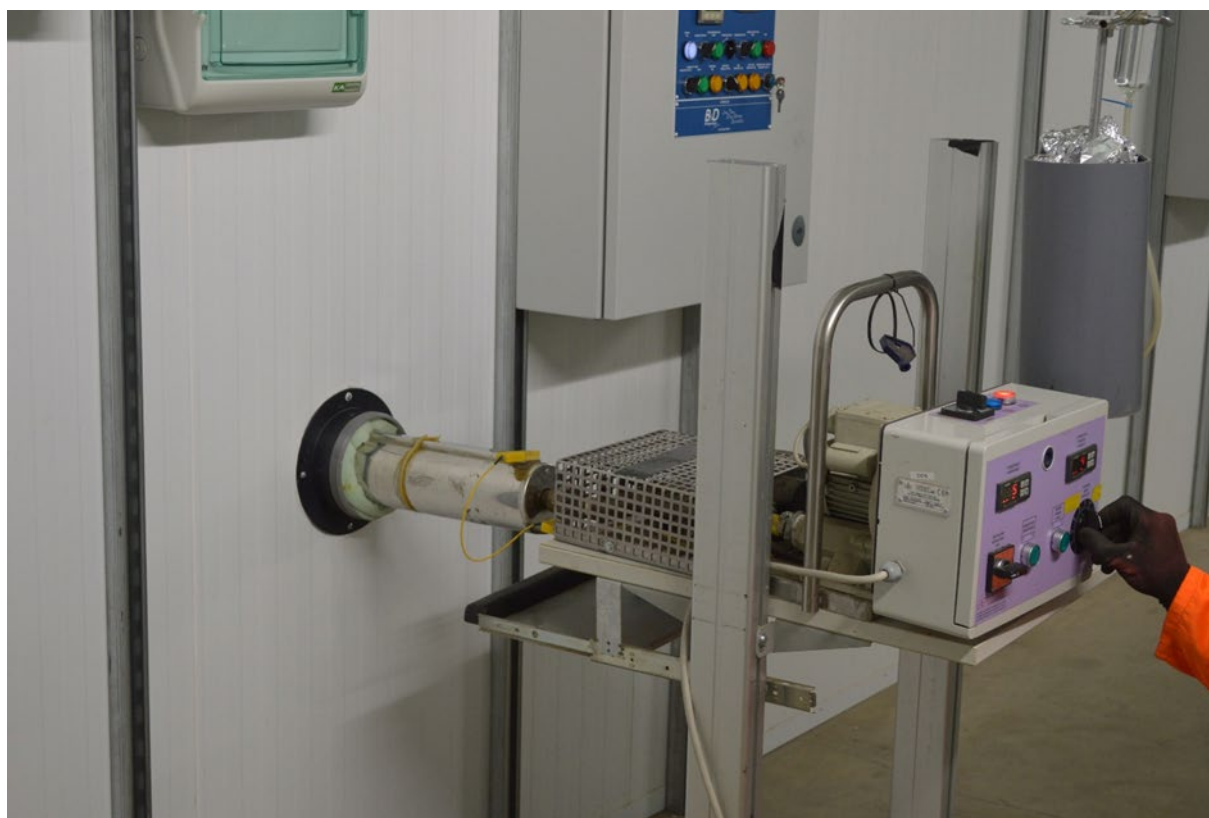
Figure 3. CEDAX Electrofog EWH-3000 for application of Mint Oil, DMN and Orange Oil.
