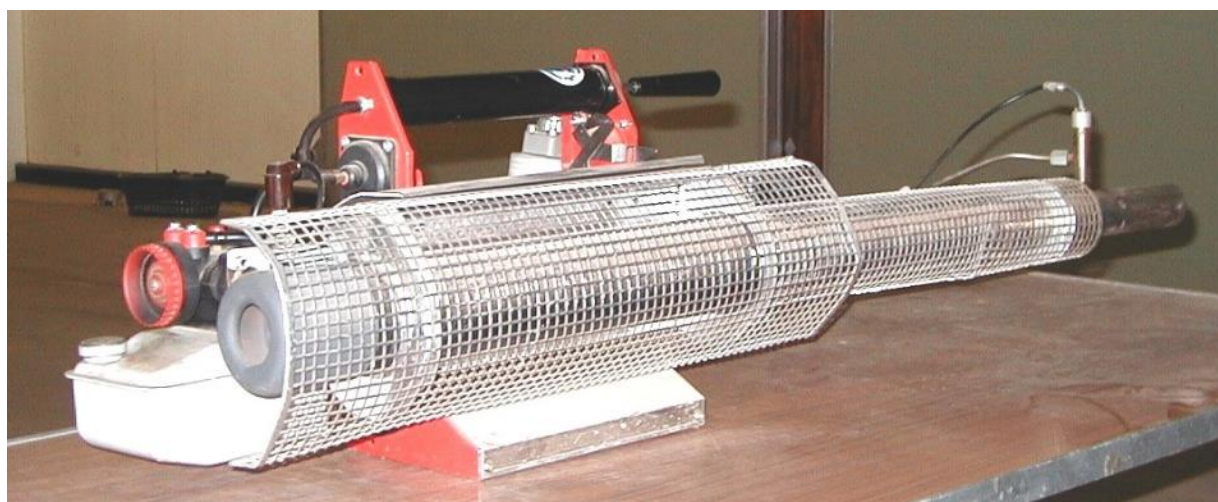
Figure 2. Swingfog SN-50 for application of CIPC as a hot fog.
